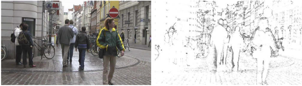
Fig. 2. Left: Still shot from one of the movies used in our experiment. Right: Corresponding image of geometrical invariant S . Non-white locations change in at least two spatio-temporal directions (brightness thresholded and inverted for better legibility).
