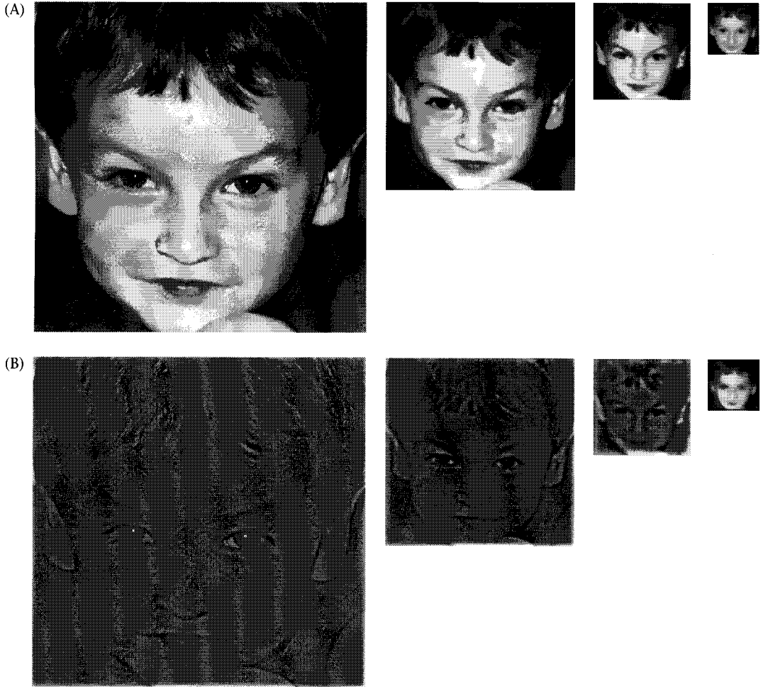
8.8 THE GAUSSIAN AND LAPLACIAN IMAGE PYRAMIDS. (A) The series of reduced images that form the Gaussian image pyramid begins with the original image, on the left. This image is blurred by a Gaussian convolution kernel and then sampled to form the image at a lower spatial resolution and size. (B) Each reduced image in the Gaussian pyramid can be used to estimate the image at a higher spatial resolution and size. The difference between the estimate and the higher-resolution image forms an error image, which in the case of Gaussian filtering is called the Laplacian pyramid. These error images can have positive or negative values, so I have shown them as contrast images in which gray represents zero error, while white and black represent positive and negative error, respectively. After Burt and Adelson, 1983.
